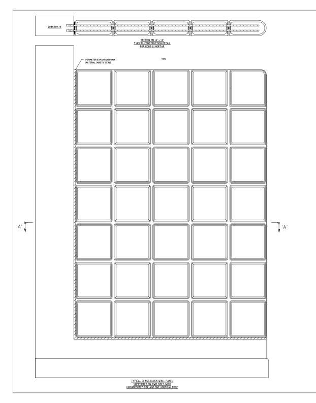
1. Glass block walls are self supporting, but not lead bearing, in addition to their own weight, they can withstand wind loads, horizontal live loads and inpact loads. A lintel provides the head for the panel to be anchored into whilst ensuring no downward pressure is placed on the glass blocks.
